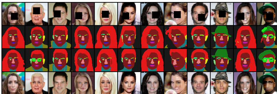
Figure 5: Segmentation from incomplete data. First row: original images from the validation set with hidden parts depicted as black squares. Second row: predicted segmentations, Third row: ground truth segmentations. Fourth row: “in-painting” – average over all images obtained during generation (with clamped visible part).
