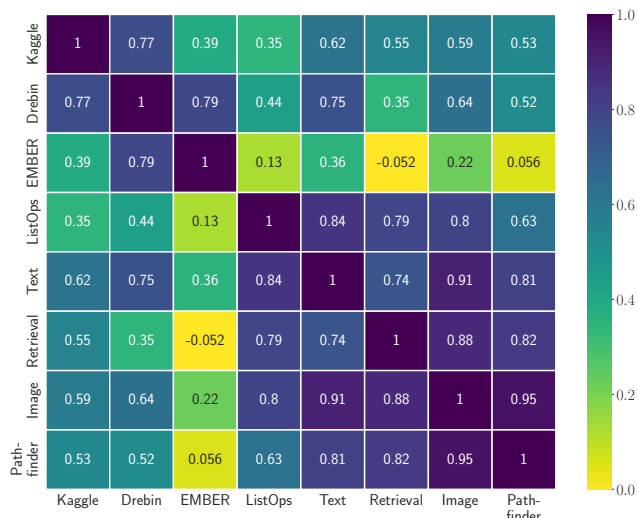
Figure 4: The correlation between Malware and other LRA tasks accuracies. While performance between LRA tasks is highly correlated with one another, they all correlate far worse with the malware benchmarks.
