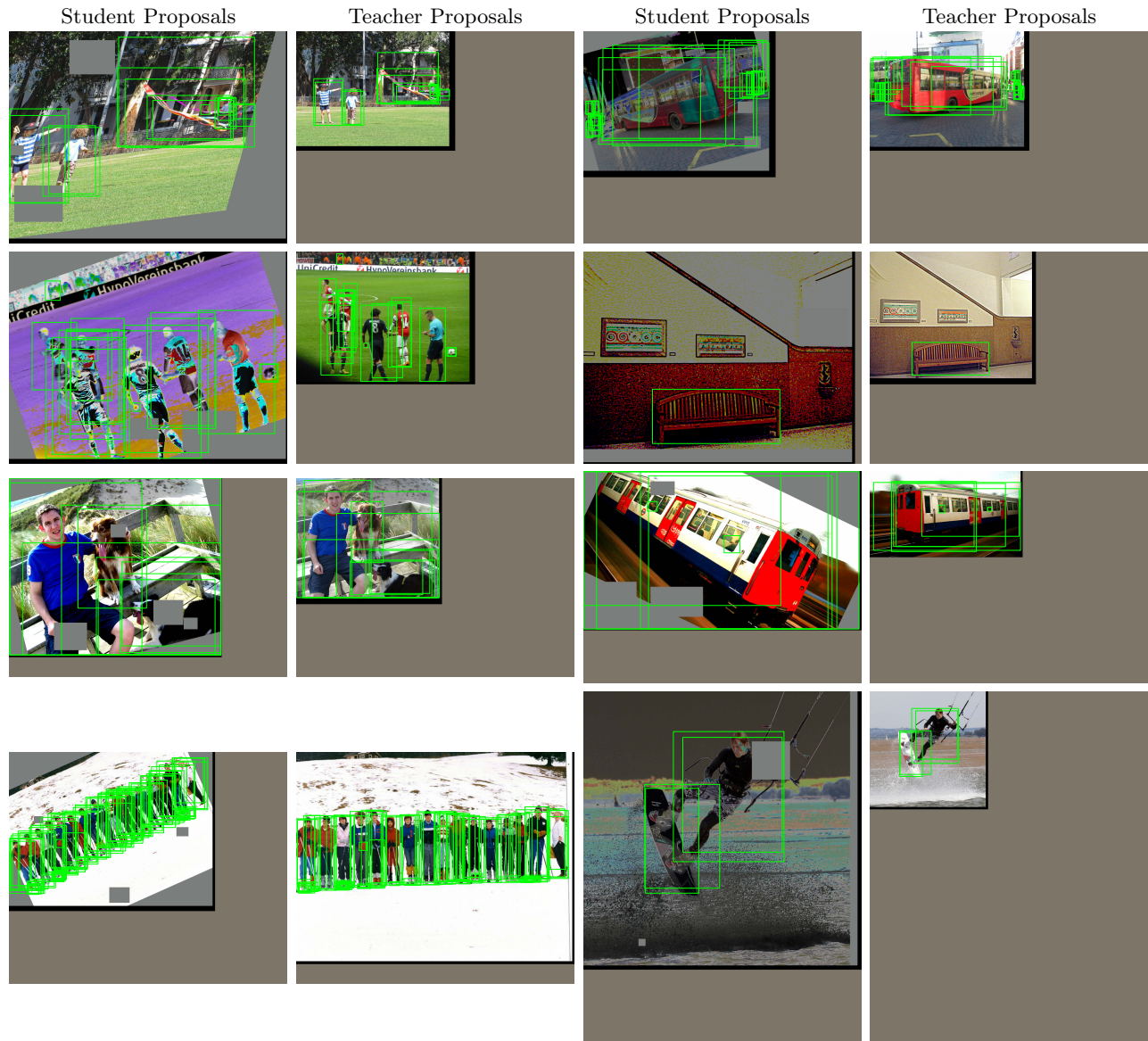
Figure 9: Visualizations of student-teacher proposals with confidence scores \geq 0.99 . A pair of student-teacher proposals is aligned between student and teacher images for the purpose of enforcing classification similarity and localization consistency. The student images are subjected to a wide spectrum of complex scale, color, and geometric distortions, whereas the teacher images undergo simple random resizing and horizontal flipping transformations as the basis for generating reliable unsupervised pseudo targets to regularize the student’s learning trajectory. This multi-stream data augmentation strategy enables the student to tap into abundant region proposals to capture diverse feature representations that would otherwise be lost with aggressive confidence thresholding associated with pseudo-labeling. Best viewed digitally.
