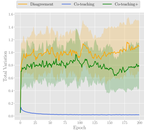
Figure 1. Comparison of divergence (evaluated by Total Variation) between two networks trained by the “Disagreement” strategy, Co-teaching and Co-teaching+, respectively. Co-teaching+ naturally bridges the “Disagreement” strategy with Co-teaching.
